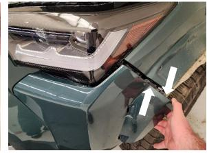
5. Remove the seven push rivets (circled 5a) securing the top radiator facia to the vehicle and remove it. With a 10mm socket, remove the 3 bolts holding the top of the grill to the core support (circled 5b). Gently lift up and out on the front clip to remove it from the vehicle and place it face down on a soft work surface.
