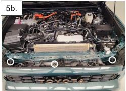
6. Use a Phillips head screwdriver to remove the three small screws securing the front fog light cover (arrowed). Stand the front clip up and remove the fog light cover starting at one end and disengaging the clips moving across.
